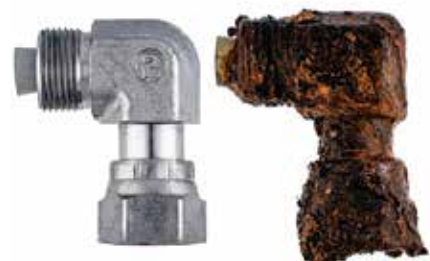
ToughShield Plus (left) and Zinc-primed (right) swivel adapters after 3,000 hours SST
